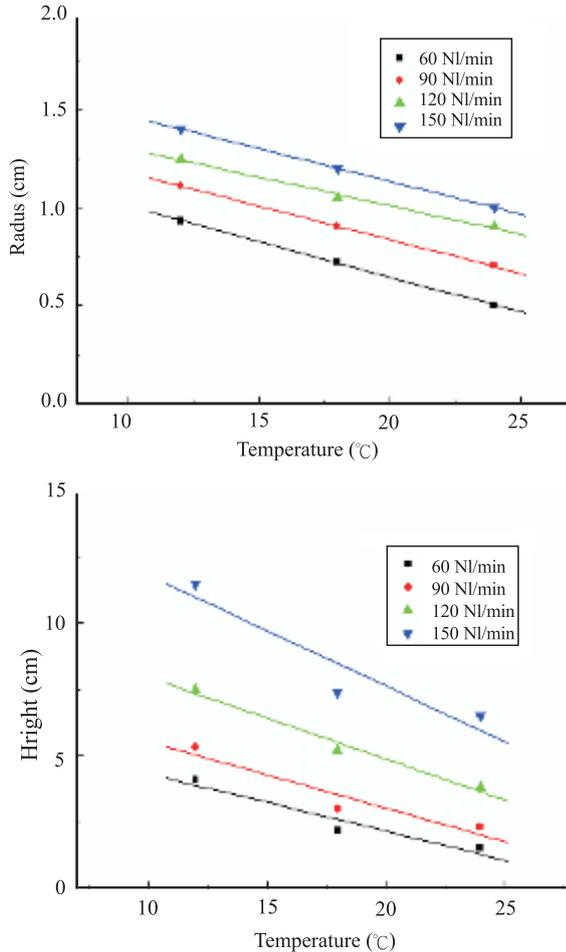
**Fig.5.** Relationship between ice dimensions and the water temperature under different gas flow rates.
