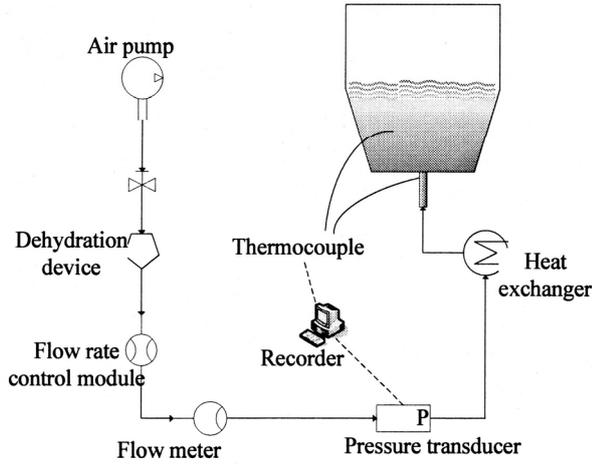
Fig.1. Schematic illustration of the water model with its gas supply system.
