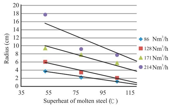
**Fig.7.** Relationship between mushroom radii and the molten steel temperature under different gas flow rates.
